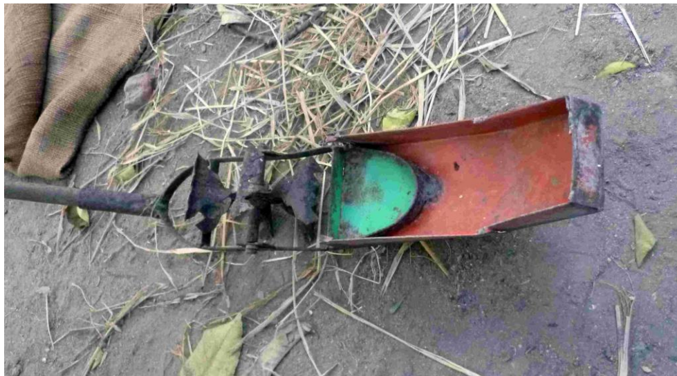
Figure 2 – Example of modified float of Raichur weeder (courtesy of Charlotte Kalkhoeven)
