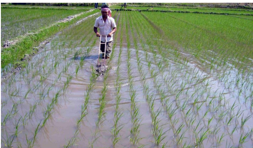
Figure 19 Paddy weeder sinking
