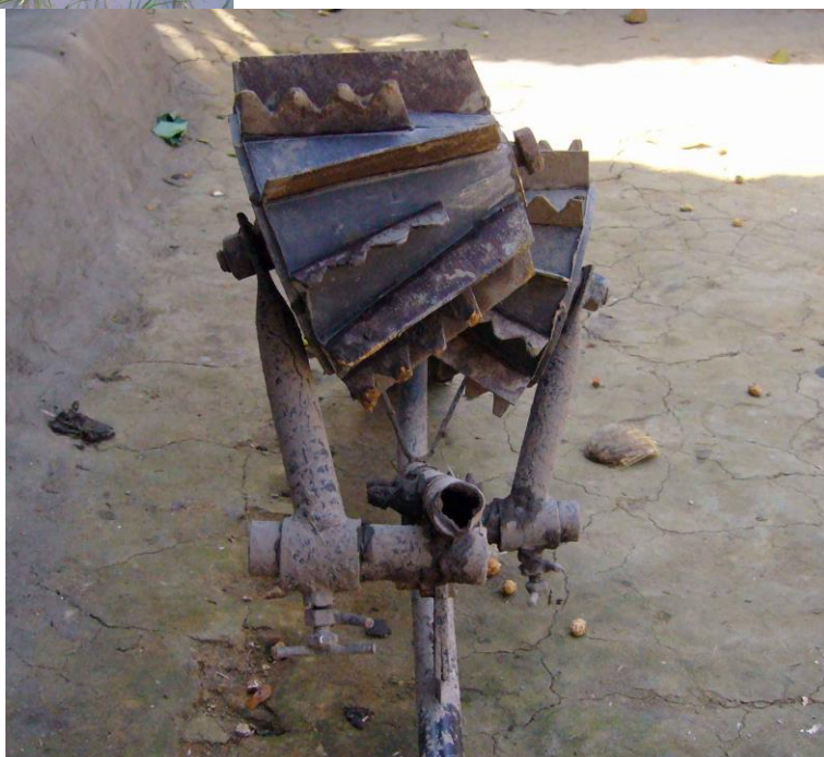
Figure 20 Details of Banabethi Cono weeder head
