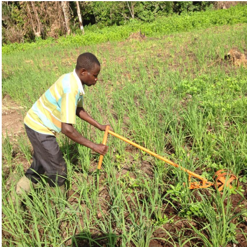
Figure 13. Farmer using wheel hoe weeder in his respective field. Source: Author's own
